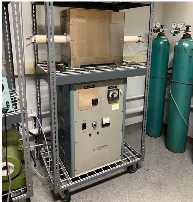
Figure 2.5.1 Tube furnace connected to oxygen gas tank used for annealing treatment.
